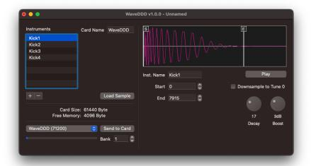
The volume is increased and the sample is run through a hard limiter. This results in these nice clipped peaks.
