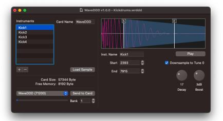
The Decay knob is limited to a value of 255, which roughly corresponds to a length of 255 \* 684 = 174420 samples at Tune = 64 and 255 \* 1024 = 261120 samples at Tune = 0.
